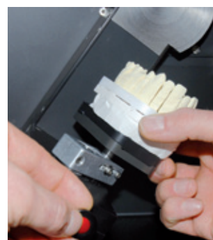
When the model is turned in the scanner, the live image and the scan also turn automatically on the monitor.
