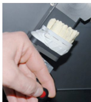
The model can be adjusted in the scanner by hand. Side effect: Waiting times during the scanning process are reduced.
