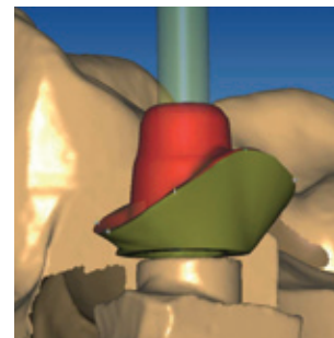
Designing the abutment using the Ceramill M-Plant software. The individual design steps are illustrated in the video tutorial on the homepage www.ceramill-m-center.com . The abutment can be fabricated in the Ceramill M-Center or using the Ceramill Motion.
