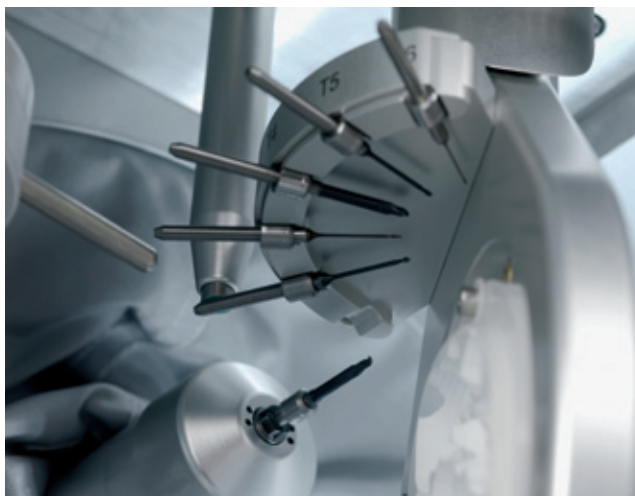
Tool magazine with automatic tool changer incl. reserve tool places.
